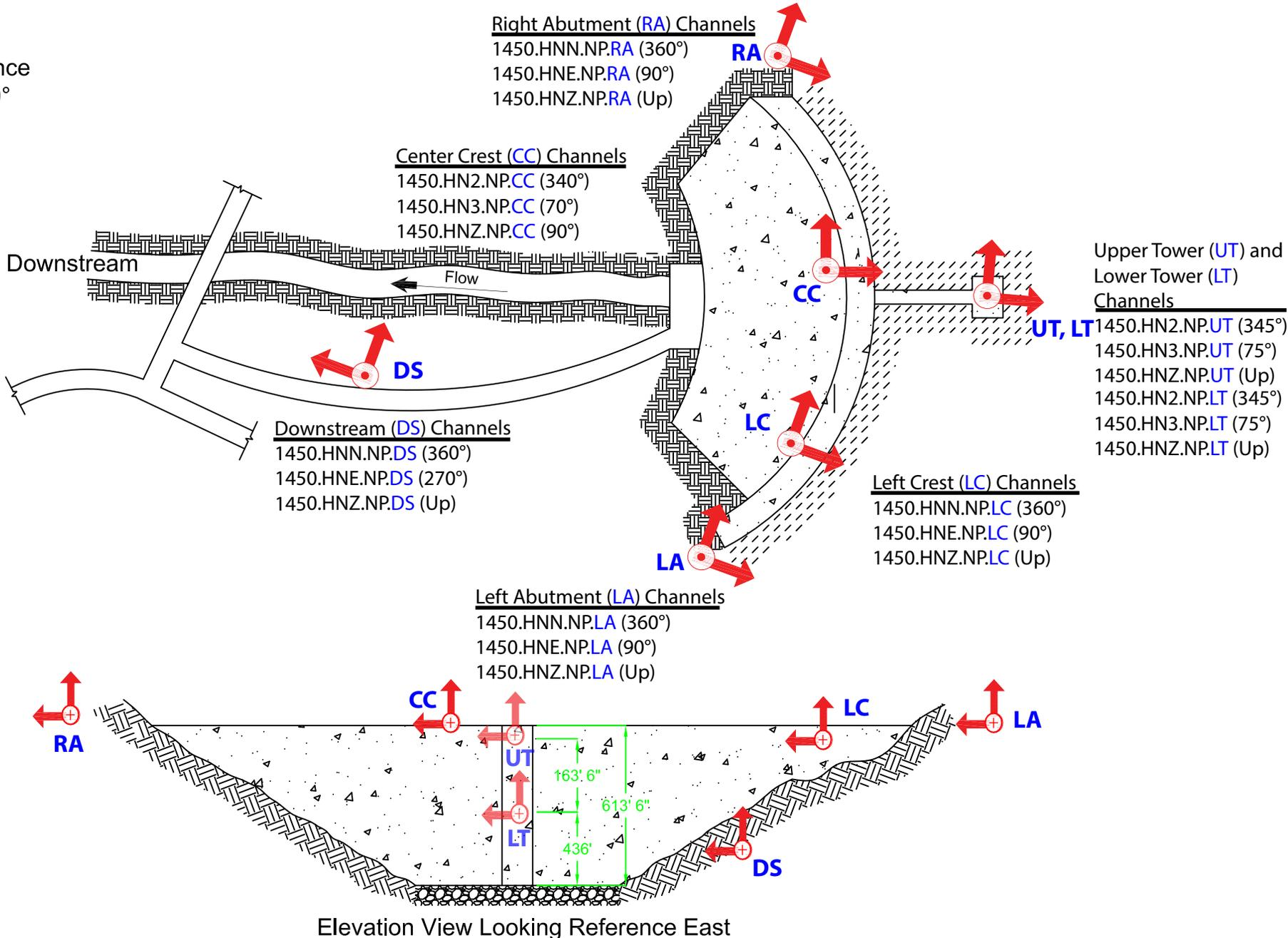
Data represented by station.channel.network.location (SCNL) and orientation from true north (i.e. 1450.HNN.NP.RA (360°))
