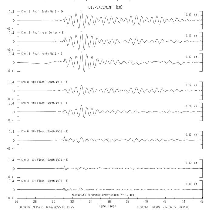
Frequency Band Processed: 5.0 secs to 40.0 Hz Automated Strong Motion Processing - Preliminary and Subject to Revision
