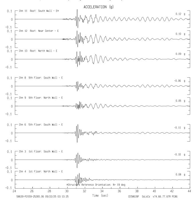
$Frequency \ Band \ Processed: \ 5.0 \ secs \ to \ 40.0 \ Hz \\ CISN/CSMIP \ Preliminary \ Strong \ Motion \ Processing - Subject \ to \ Revision$
