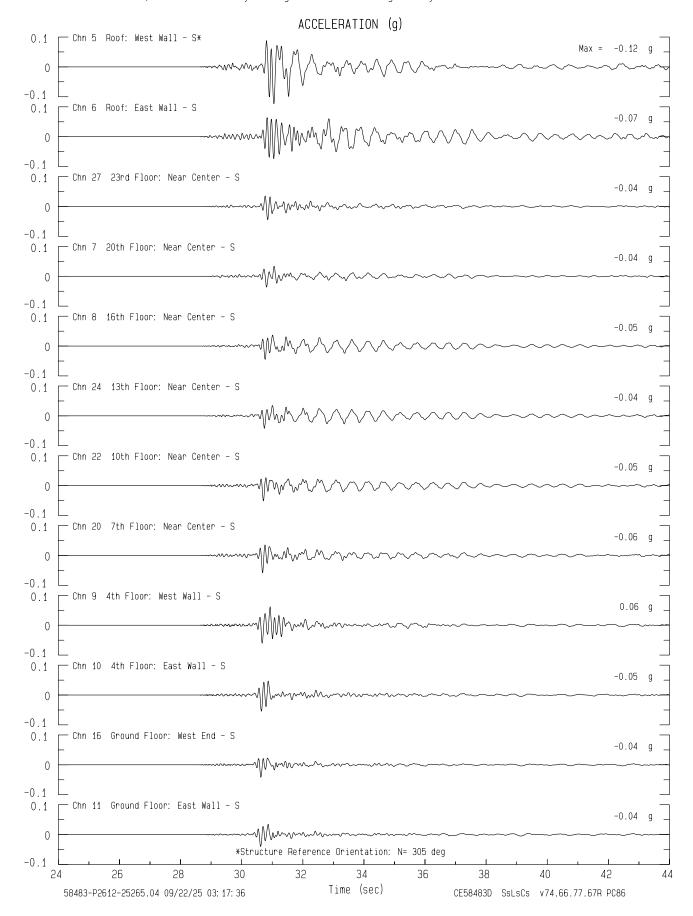
Frequency Band Processed: 5.0 secs to 40.0 Hz CISN/CSMIP Preliminary Strong Motion Processing - Subject to Revision
