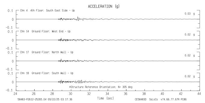
Frequency Band Processed: 5.0 secs to 40.0 Hz CISN/CSMIP Preliminary Strong Motion Processing - Subject to Revision
