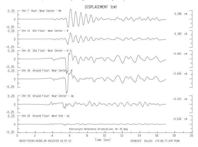
Frequency Band Processed: 5.0 secs to 40.0 Hz Automated Strong Motion Processing - Preliminary and Subject to Revision
