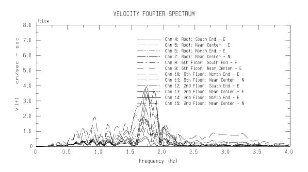
Frequency Band Processed: 5.0 secs to 40.0 Hz Automated Strong Motion Processing - Preliminary and Subject to Revision
