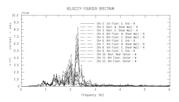
Frequency Band Processed: 5.0 secs to 23.0 Hz Automated Strong Motion Processing - Preliminary and Subject to Revision
